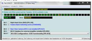
After coding, head-unit must be reset. On most head-units by long-pressing (about 20 seconds) of the ON/OFF key.
