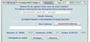
In Byte 19 set bit 4 to "Rear View Camera installed"
